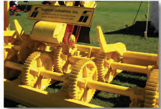
Split bullwheels allow for simple and fast replacement.
