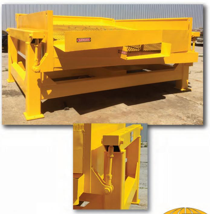
Fulghum's rotary screens separate out over size chips and fines producing near perfect chip grading; chips uniform in size, free of sawdust and splinters.
